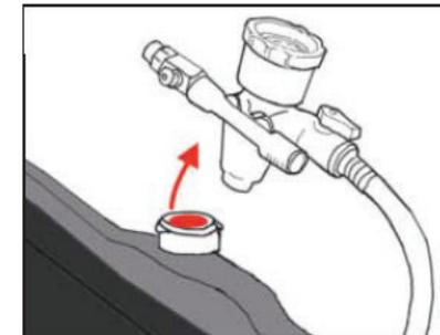
6. Remove the radiator air bleeder from the radiator opening and replace the radiator cap.
